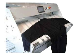
folding templates and air blasts. The measuring of each item combined with a large primary fold section allows operators to process mixed batches containing a wide range of sizes.
