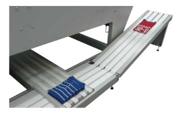
predetermined height, a retractable conveyor neatly transfers the items onto the final delivery belt.
