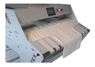
Once a stack reaches its predetermined height, the unit neatly transfers it onto a final delivery conveyor belt located at either the left or right side of the unit and delivers it to either the front or the rear of the machine.
