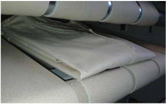
are made by air-assisted reversing belts. A neatly folded package is obtained by continuously pressing the items between belts as they move through the machine. Top-quality stretch belts ensure that the thickness of the linen does not affect folding quality.
